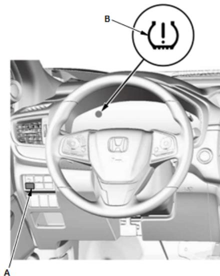
1. Make sure the tires are inflated to the specified tire pressure listed on the doorjamb label.
